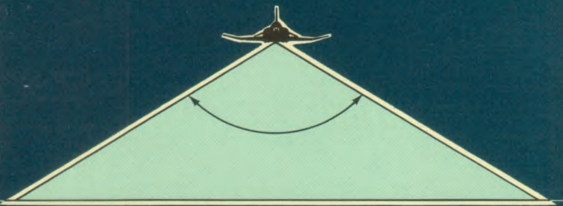
EO Wide Angle, Vertical has 140° FOV
